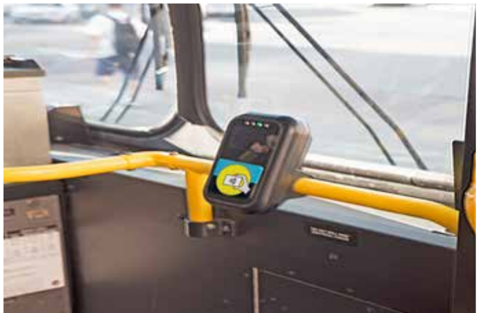
Figure 3: Ventra Electronic Fare Card Mobile Validator mounted inside a Pace Bus.
